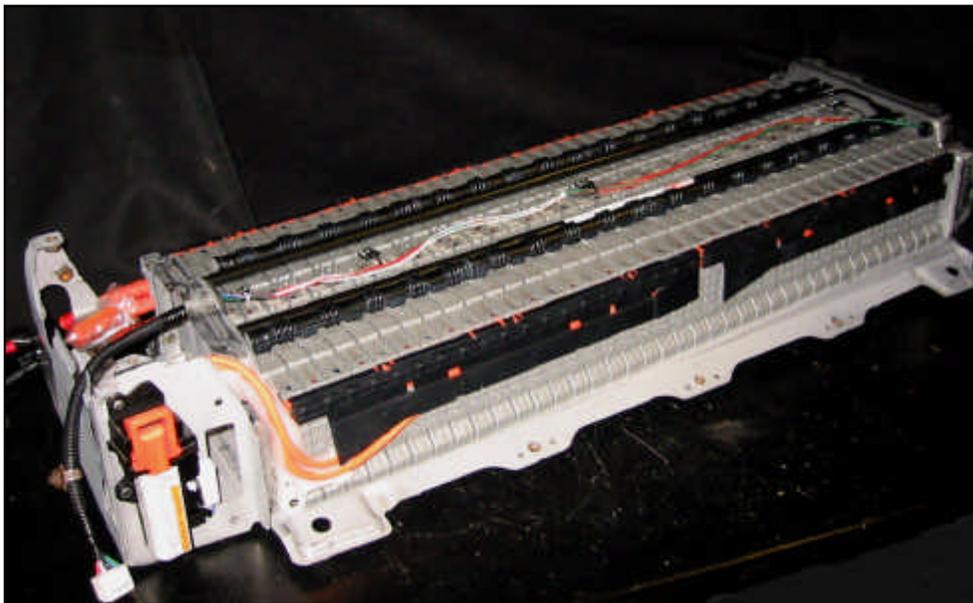
*This Prius battery pack (shown with cover removed) will be used in parallel with our Landrover Td5 diesel engine.*
